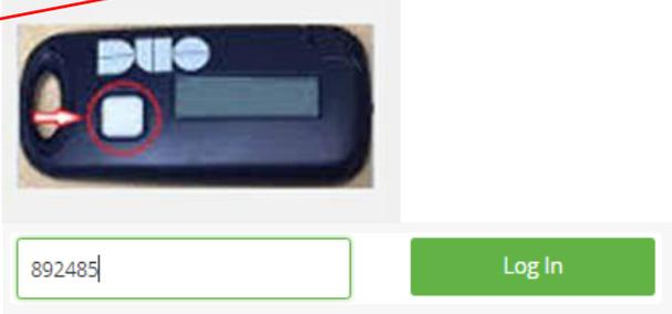
The image shows a physical Duo token, a small black device with a white button and an LED screen. A red arrow points to the white button. Below the token is a screenshot of the login page showing a text input field containing the passcode "892485" and a green "Log In" button.
